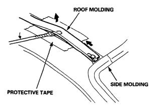
Pull and slide the roof molding, then detach the bracket on the end of the roof molding from the pin.
