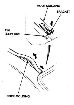
3. Pull the roof molding up, detach the bracket from the pin, then remove the roof molding.
